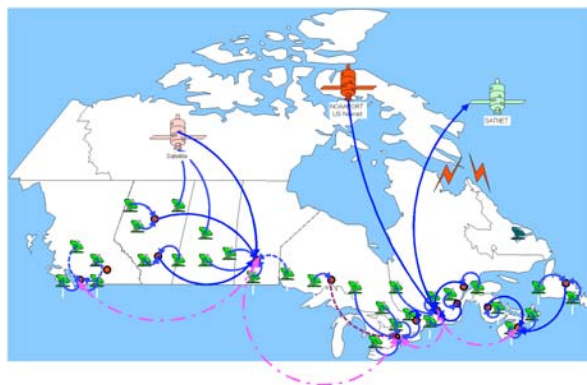
Figure 1: Data topology of the Canadian National Radar Network. The radar icons indicate the location of the radars. Solid lines indicate existing pathways for the volume scans and the dashed lines indicate future radar installations. Dash-dot lines indicate inter-Regional data flow paths. Note the ingest of NEXRAD data at the Canadian Meteorological Centre and the subsequent re-transmission to the Regions via SATNET.
